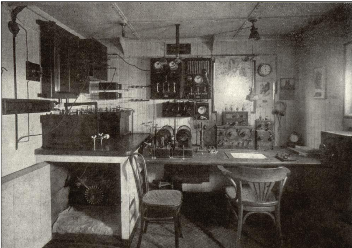
An early, 1.5 kilowatt Marconi transmitter. Similar equipment may have been installed in the top floor of the Tower.
