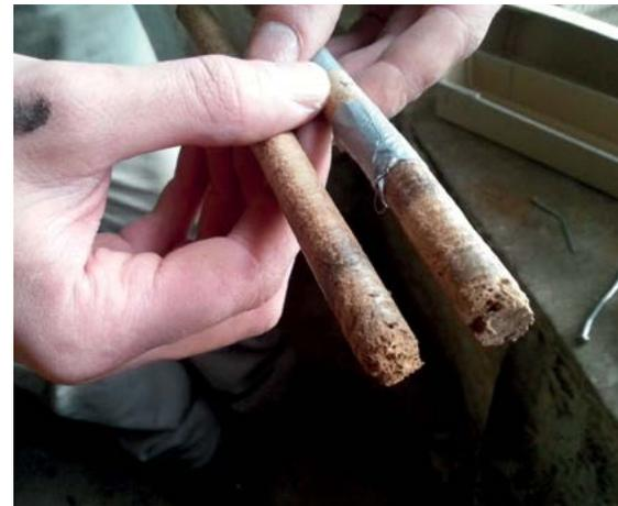
Two of the timber cores taken from a joist allowed us to date the low end to the 1420/21 felling season.
