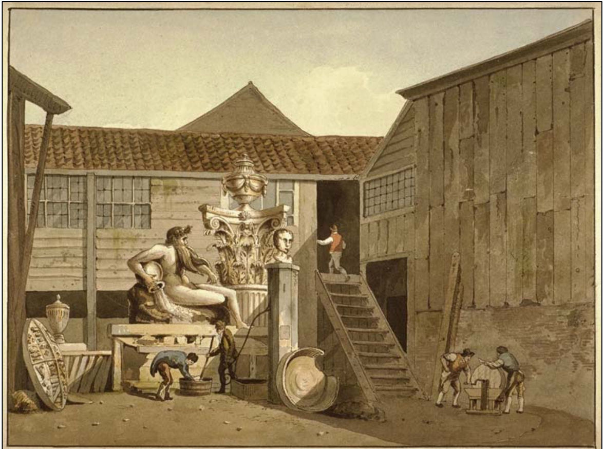
A contemporary watercolour showing the yard of the Coade manufactory in Lambeth c1800. The River God (as at Ham House, Richmond) is prominently displayed, as is the royal coat of arms hinting at Mrs Caode's Royal Warrant. Workmen grind grog, and mix the raw formula in a tub.
