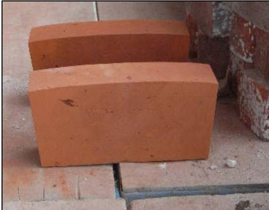
Dark and light red 'rubbers' were specially made to match the colour variation of the originals. The bricks to be used for replacement in the turret skins (like these) were rubbed to shape off-site at Bulmer Brick and Tile Company.
