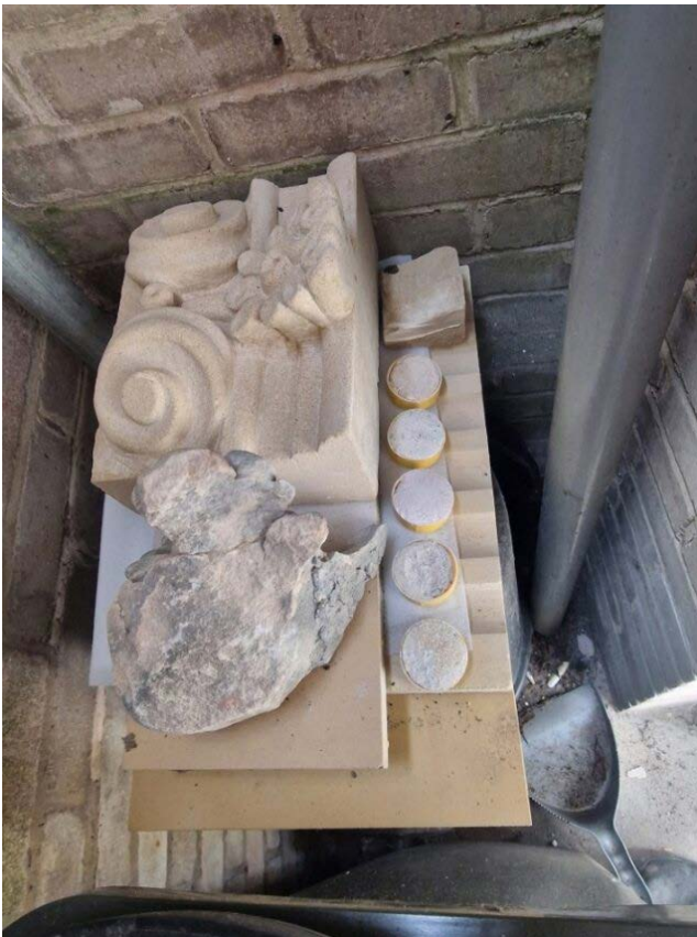
Clockwise from top left: the NW corner masonry after removal of inappropriate cementitious repairs and after repair; the Music Room shrouded for repair; lime samples were carefully matched to the colour of the stonework.
