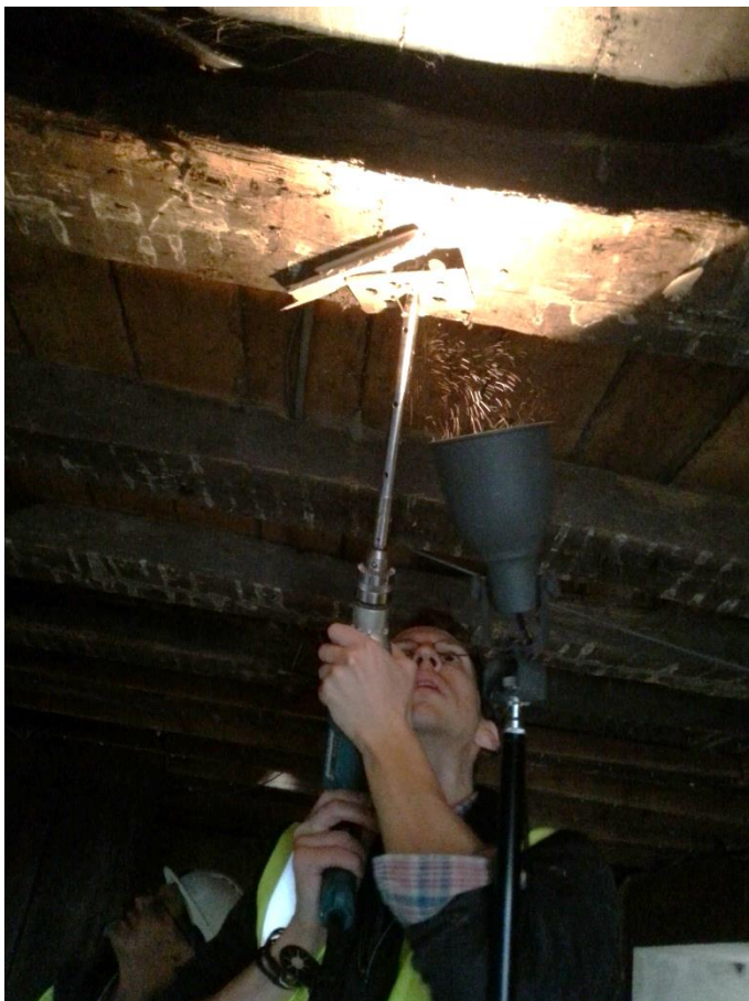
Drilling timber cores in the rear kitchen (above) and snug (below) in 2014.
