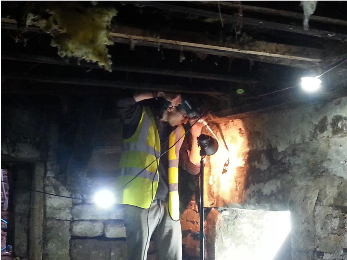
Drilling timber cores in the rear kitchen (above) and snug (below) in 2014.
