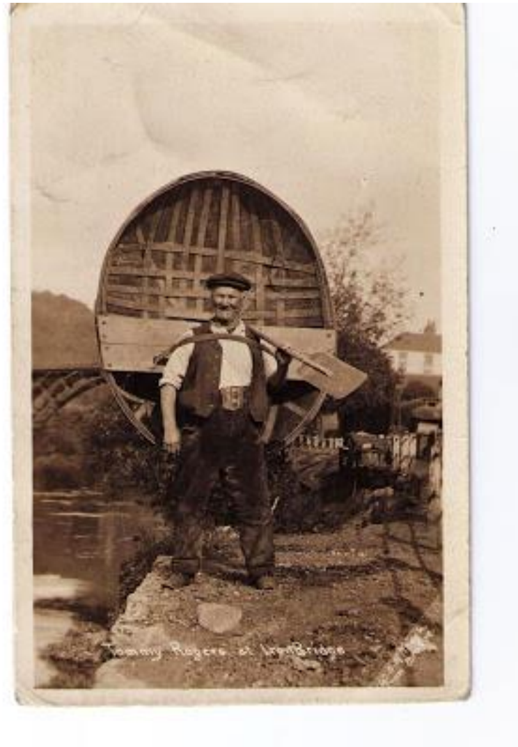
Tommy Rogers, born c.1845, coracle maker of Ironbridge. A coracle is a small, lightweight boat with a loosely woven frame traditionally covered in animal hide, but in more recent times they are made from calico, canvas and coated with a substance such as bitumen.
