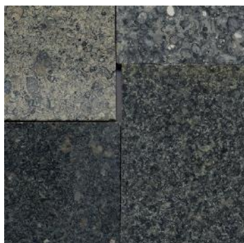
Examples of Purbeck stones: clockwise from left: some Purbeck marbles; Thornback; Grub, Freestone; Downsvein. The limestones vary in hardness, colour and fossil content according to their
