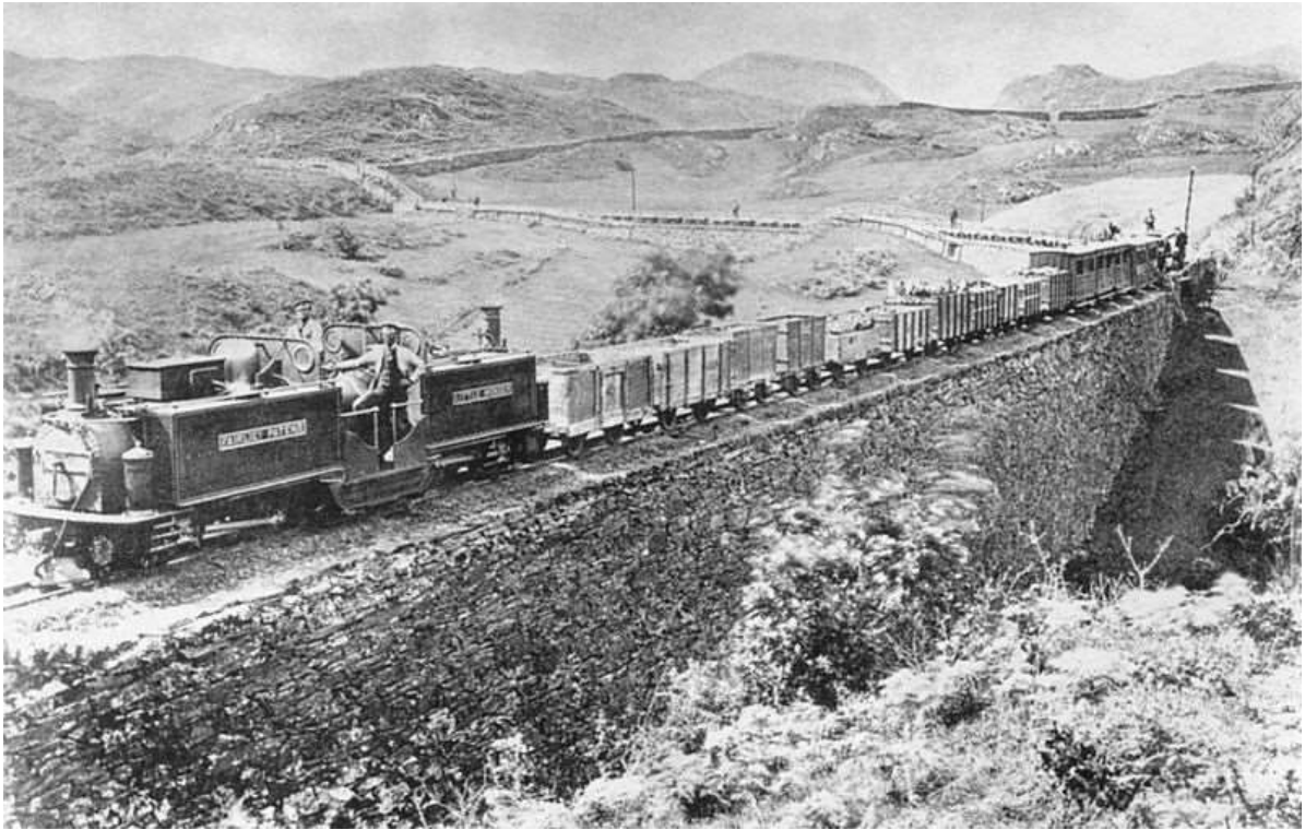
Ffestiniog Railway's first double Fairlie locomotive "Little Wonder" with long mixed train rounding Cei Mawr in 1871, pulling a very long train loaded goods wagons, passenger carriages, and empty slate wagons.
