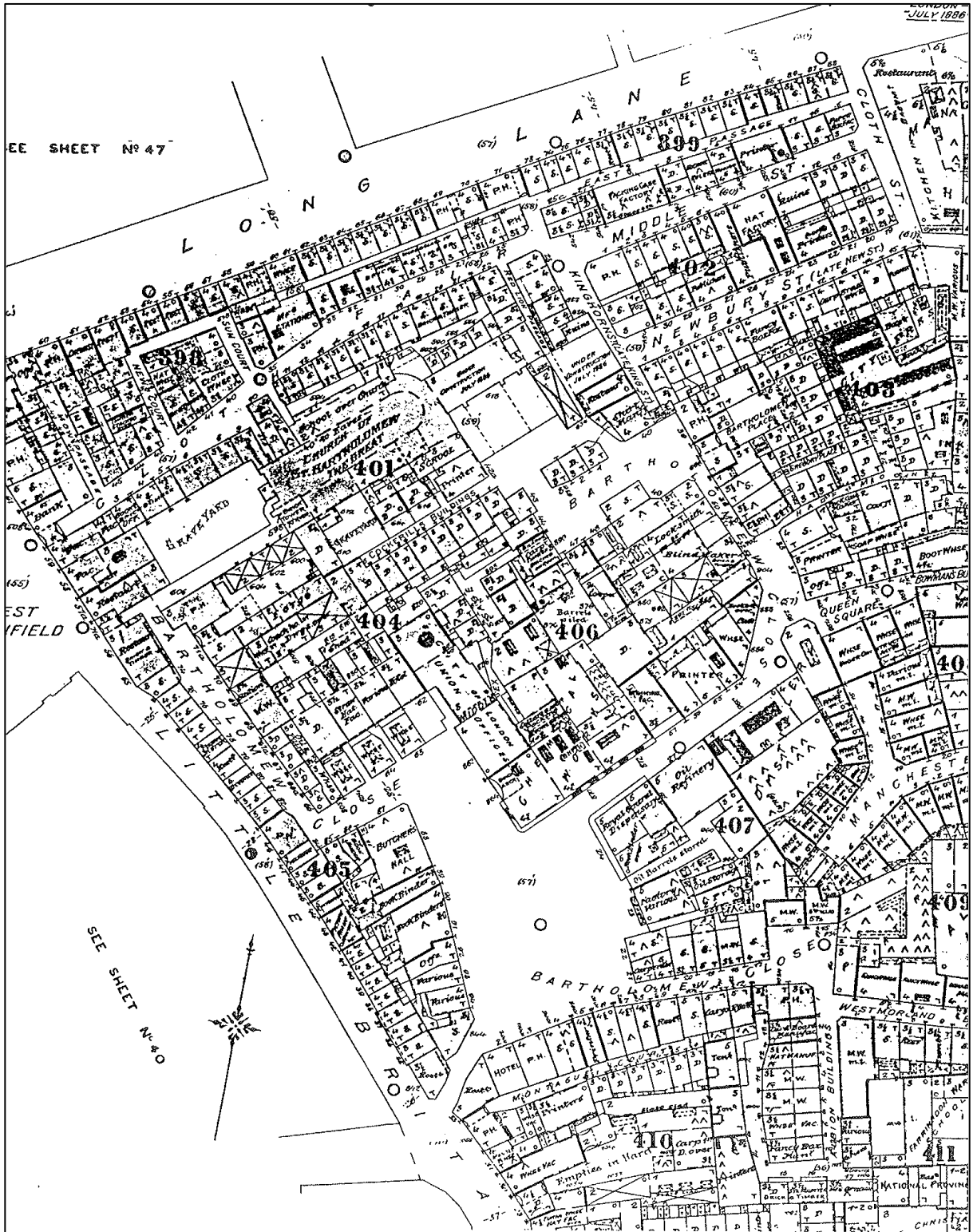
An insurance map of 1886. Notice how the use of the buildings is noted, and the materials of which they are built, if those could be a fire risk. The restoration of the church has just begun, work being carried out in the Lady Chapel.
