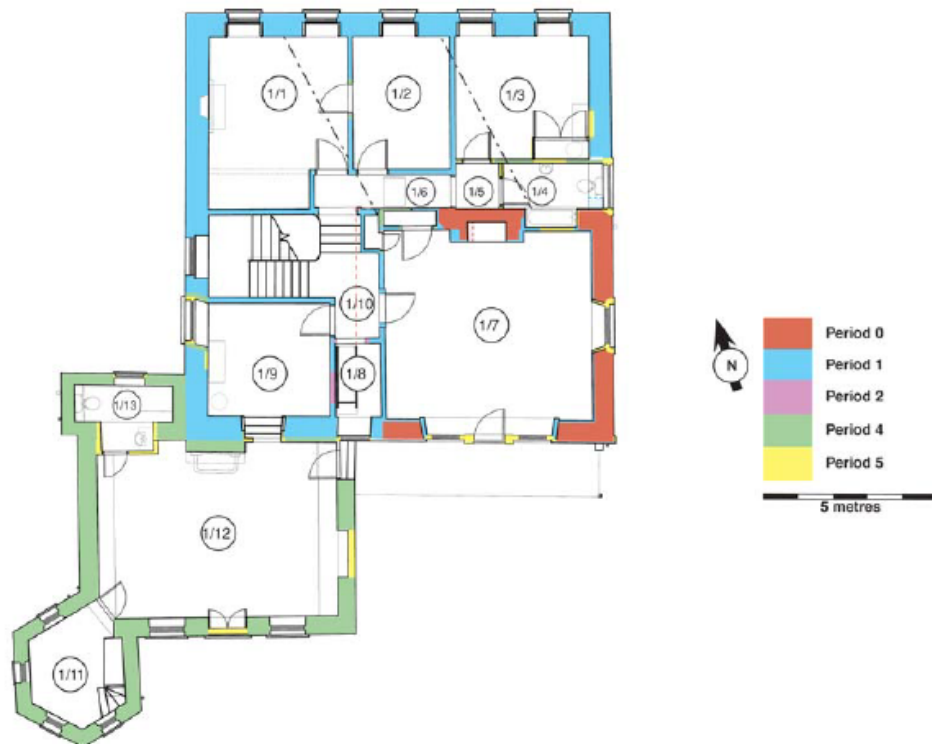
Figure 3: Belmont: Phased plan of first floor; chain lines represent the first floor bridging beams
