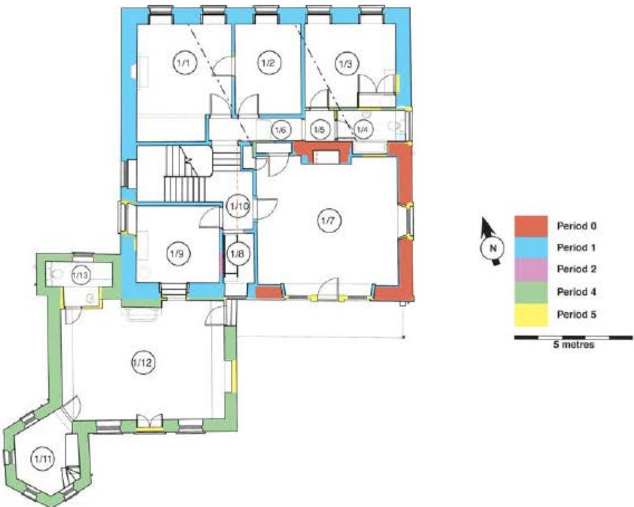
Figure 3: Belmont: Phased plan of first floor; chain lines represent the first floor bridging beams
