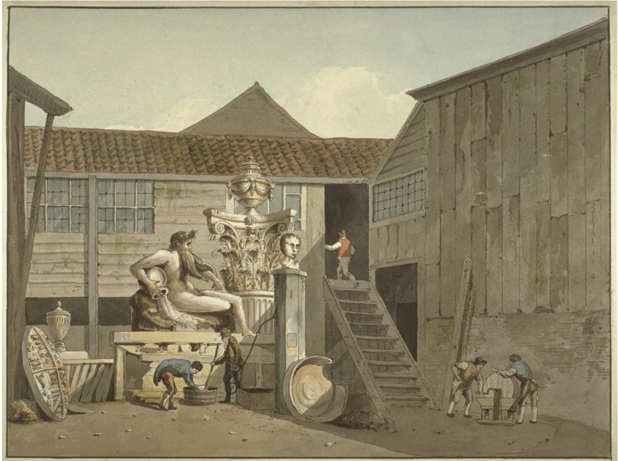
This watercolour shows the yard inside the Coade manufactory, behind the showrooms. Two men are grinding the grog on a wheel; others are mixing clay in a tub. A River God awaits collection, as does a Royal coat of arms (Coade held the Royal Appointment to both George III and George IV).
