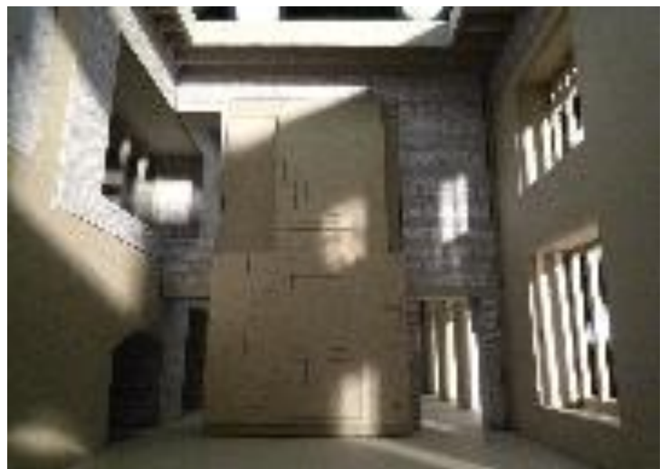
The latest technology was used to help develop the scheme. An 'artificial sky' at the Bartlett School of Architecture, University College London, here dwarfs the model of the castle. The computerised lamps enable the light to be simulated for any time of year or day, in all weather conditions, to help finetune the placing of windows and openings. As seen in the two examples below, the simulations proved remarkably accurate of the end results (left: first floor, kitchen area; right: the garden court).
