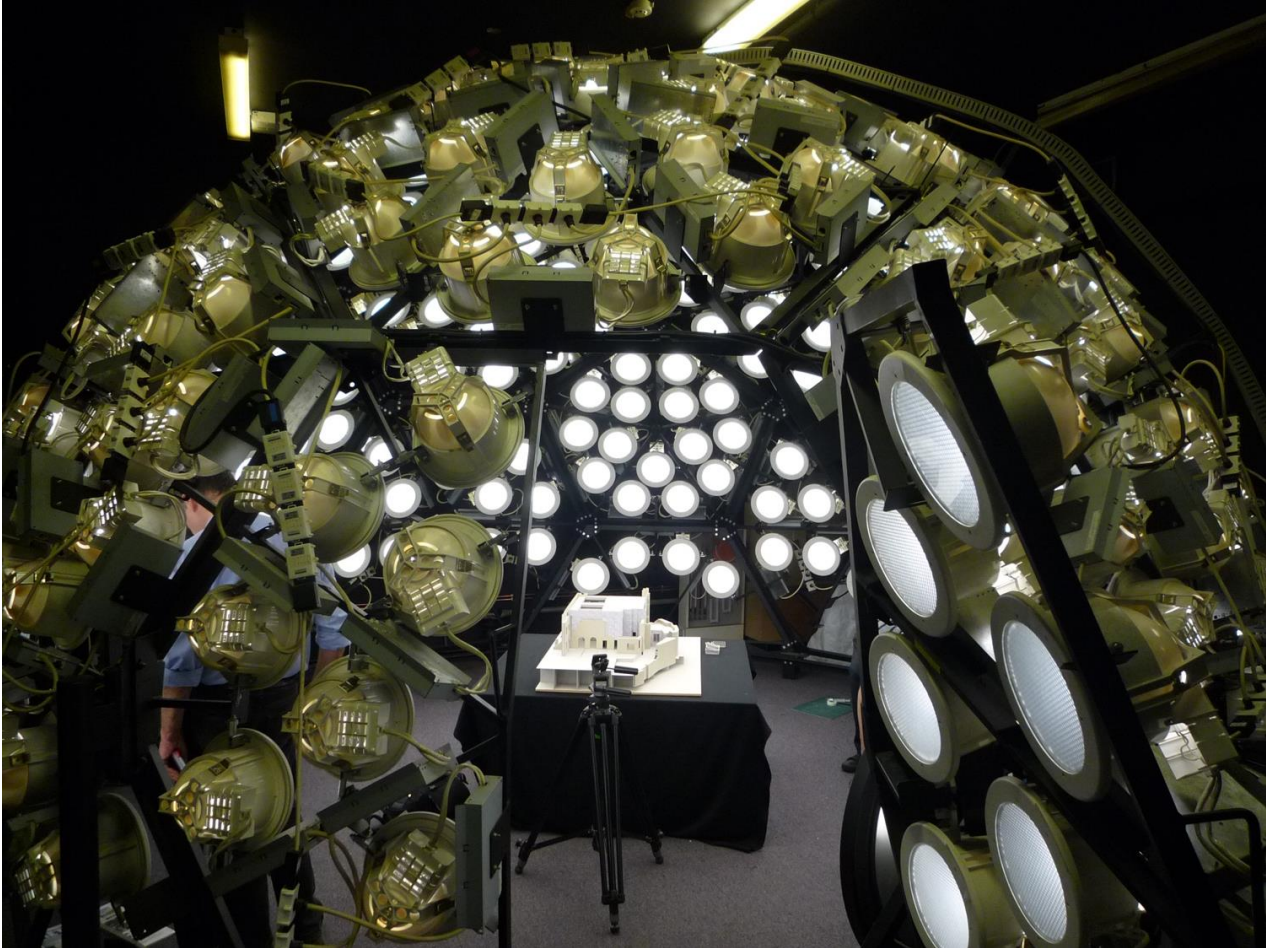
The latest technology was used to help develop the scheme. An 'artificial sky' at the Bartlett School of Architecture, University College London, here dwarfs the model of the castle. The computerised lamps enable the light to be simulated for any time of year or day, in all weather conditions, to help finetune the placing of windows and openings. As seen in the two examples below, the simulations proved remarkably accurate of the end results (left: first floor, kitchen area; right: the garden court).
